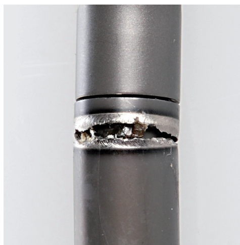
Figure 5. Nail breakage at the welding seam in the PRECICE device in the patient shown in Figure 4.
