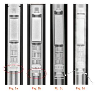
Plain radiographs of different internal mechanisms in retrieved Precice nails. a) Radiograph of early P1 design, with a longer frame compared with the rest of the designs. b) Radiograph of the later P1 design with a smaller frame. c) Radiograph of P2 design with an arrow showing the metal rings close to the actuator pin. d) Radiograph of P2.1 design with an arrow showing the metal rings.
