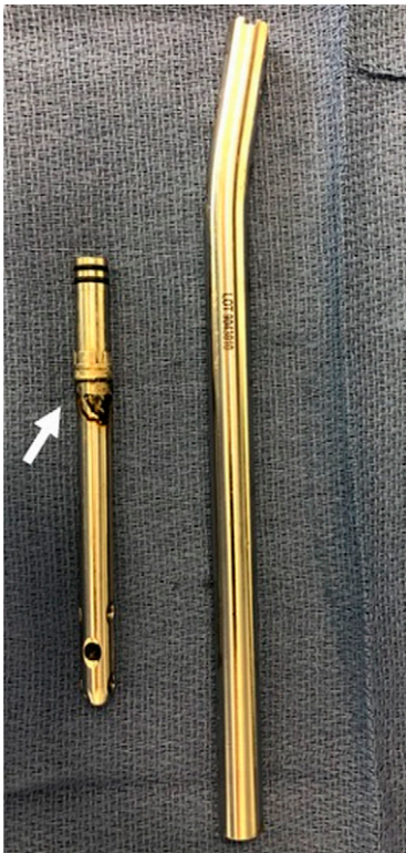
Fig. 4 The distal component (left) and the proximal component (right) of the nail are shown. White arrow indicates corrosion at the component interface.
